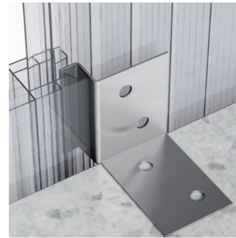
PLATE DETAIL OF INTERMEDIATE PLATFORM.
