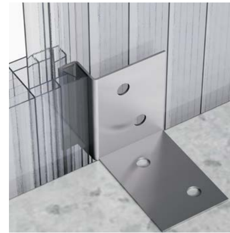
PLATE DETAIL OF INTERMEDIATE PLATFORM.
